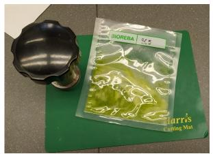
Figure 2. Sample homogenization in the extraction buffer (Photo: G. Barać)
