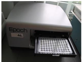
Figure 4. Reading of results by BioTek Epoch type spectrophotometer (Photo: G. Barać)
